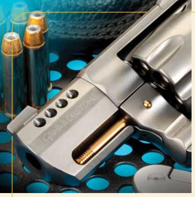
The original barrel is replaced with a Gemini Customs "Ultimate" 12-angle profiled barrel (above) after considerable effort to make sure the replacement is lined-up and top-dead-center. Gemini Customs uses Armor Guard "Copper" PVD plating for an eyecatching and practical accent. The hammer (below) is centered and shimmed while the cocking spur serrations are cut at 25 LPI.
